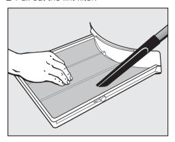
■ Wipe the lint off the filter with your hand (do not use any sharp objects!) or use a vacuum cleaner with the nozzle attachment (supplied with the vacuum cleaner).
